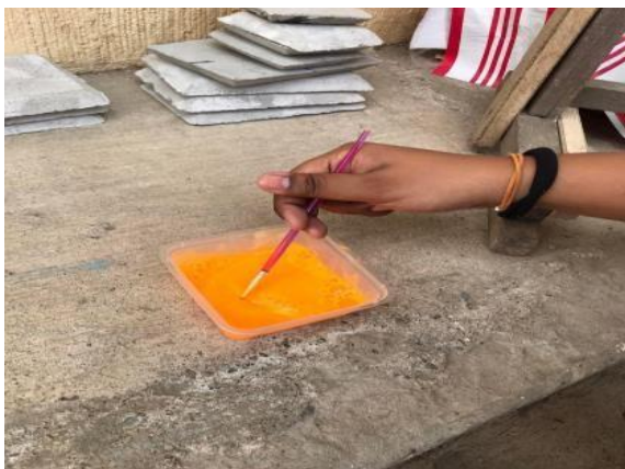
Fig. 5. Mixing of Epoxy Resin and GiD Powder
