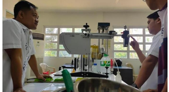
Fig. 9. Skid Resistance Number Tester
