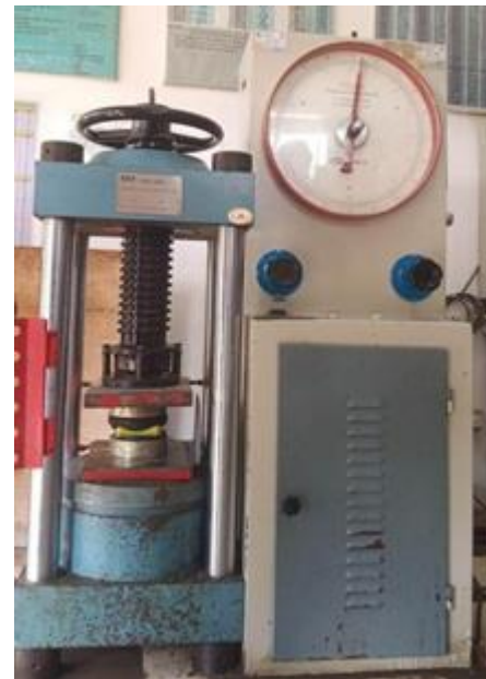
Fig. 10. ASTM D4280 Compressive Strength Machine
